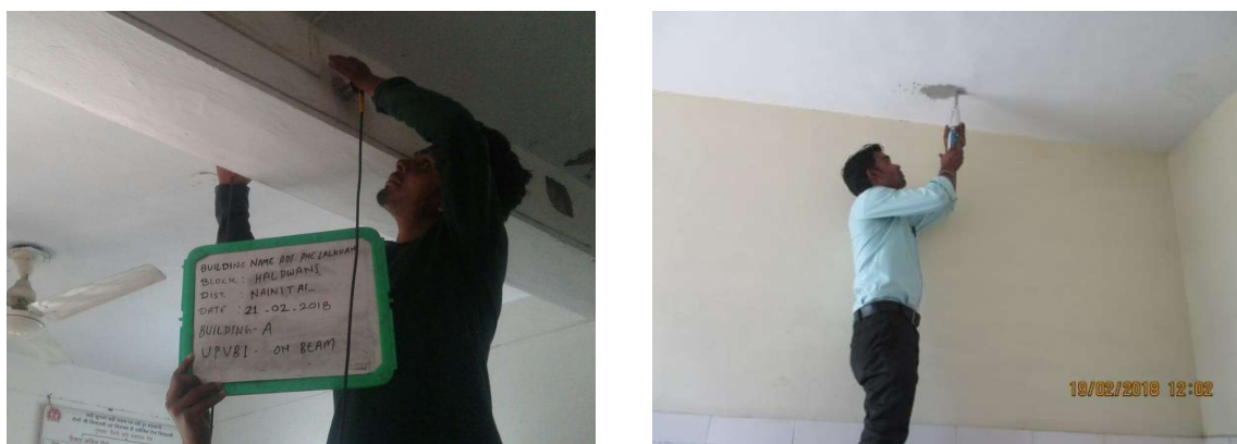
Figure B.5: USPV & Rebound Hammer Test being conducted in Masonry Building
