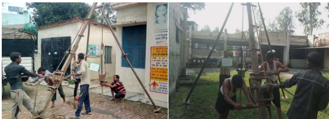
Figure B.7: SPT & DCPT being carried out on site
