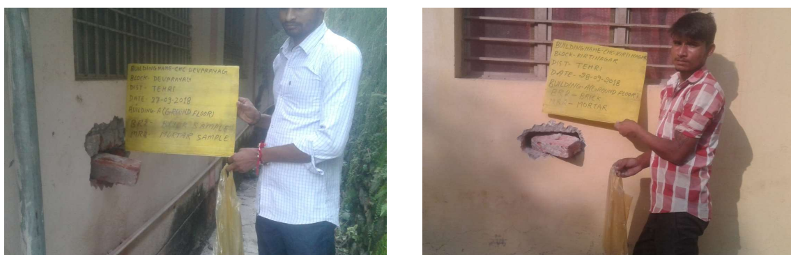
Figure B.4: Masonry Unit & Mortar Samples being collected from site
