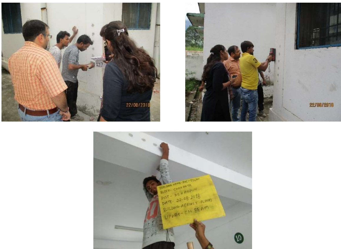
Figure B.10: Rebound Hammer, Ultrasonic Pulse Velocity and Rebar locator Tests being conducted on sites
